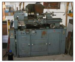
converted for single phase use with a Transwave converter. The converter is the large blue box shown in top right-hand corner of the picture.
